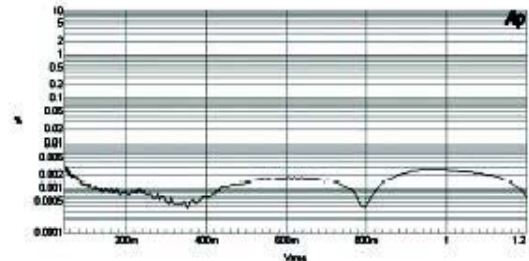
CCIF & IMD distortion – 14 kHz and 15 kHz
