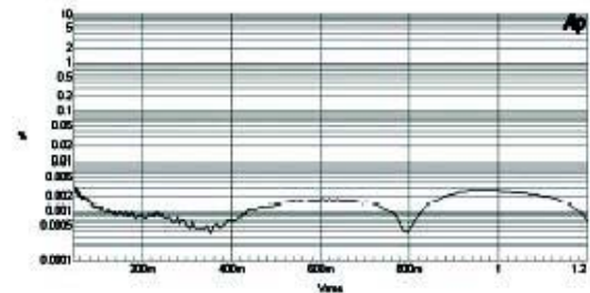
CCIF & IMD distortion – 14 kHz and 15 kHz
